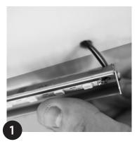
Ensure mounting surface is clean and dry. Drill wire exit hole through mounting surface. Thread wiring through hole.
